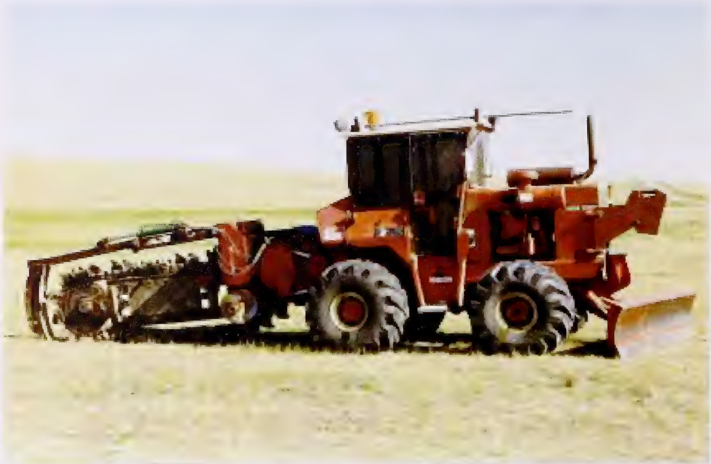
Photo 50 Low impact chain wheel ditcher.
